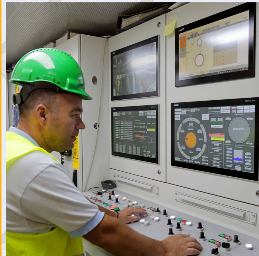
TBM "ATHENA" - Steering chamber.
